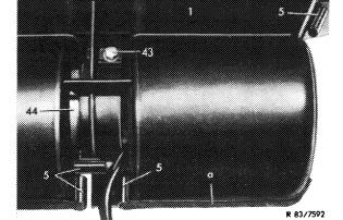
Evaporator housing with cooling blower
