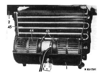
Layout of evaporator and cooling blower in evaporator housing
