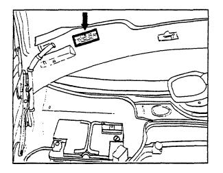
Figure 2 Model 124 (except 124.034/036) On hood crossmember above battery.
