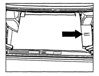
Figure 4 Model 124.036 On battery compartment cover, visible with floor mat lifted.
