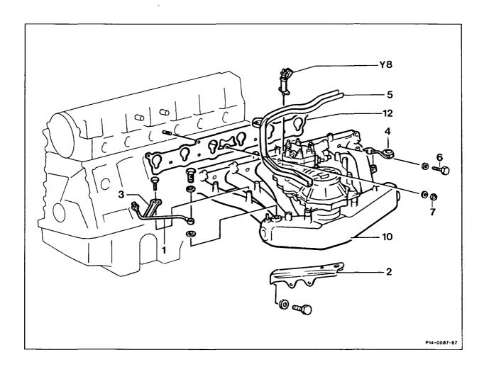
Ground cable at battery ..... disconnect, connect. Engine compartment panel ..... take off, fit on. Plastic rail (5) for engine wiring harness ..... remove, install. Mixture control unit with air guide housing ..... remove, install (07.3-1668). Holder for starter cable (4) ..... detach, fit on. Vacuum connections at intake manifold and throttle valve body ..... pull off, fit on. Vacuum line (1) for brake booster with holder remove, install.
