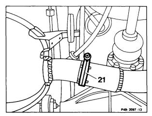
New tail silencer (9n) ...... position with plug connection exactly over the removed exhaust system and mark pipe length of new tail silencer on the removed exhaust
