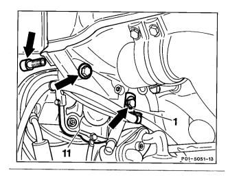
9 Extract oil from the reservoir of the power steering pump with the handpump, special tool 112 589 00 72 00 for extracting oil.
