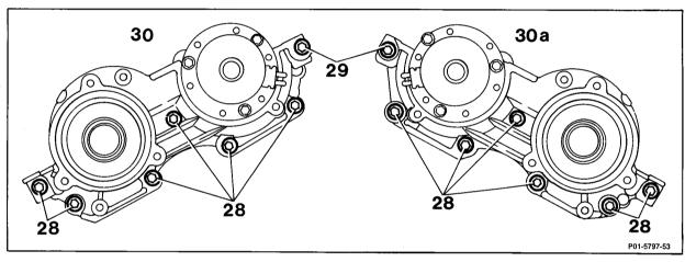
28 M8×25 hexagon socket bolt + washer 29 M8×35 hexagon socket bolt + washer
