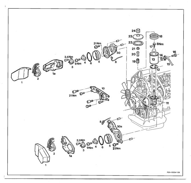
Bracket (10) of actuator ...... detach, attach (21 Nm) (step 1).
