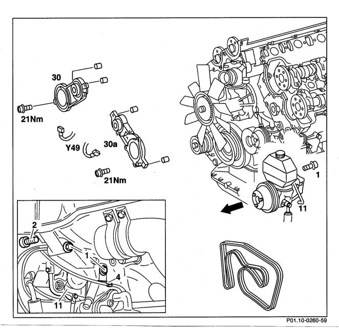
Left front cover (30a) on version with power steering pump: .....
