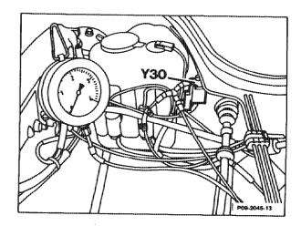
15 Test exhaust backpressure at exhaust manifold, only (SA) California.
