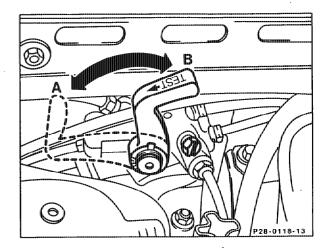
13 Test exhaust level under load. If the specified exhaust levels under load are not achieved, set injection pump to the upper tolerance limit on the pump test stand.
