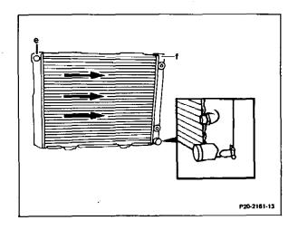
On model 201.128 the crossflow radiator with turbulence plates in the cooling pipes is installed below the radiator bridge. It is held in the radiator bridge at the top by two retaining lugs (arrows).
