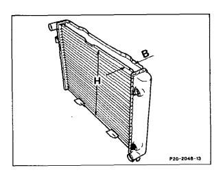
Drain plug on engines 601 and 602 arranged vertically, on engine 603 arranged horizontally.
