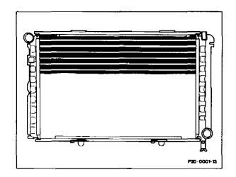
The bottom radiator position is installed as standard on models 124.125/185 effective 01/90. The round tube radiator has been modified in accordance with the altered installation conditions.
