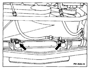
The mounting points at the body and the fan cowl version differ according to the various radiator designs.
