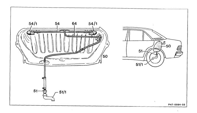
The vent system in the fuel tank (50) consists of a central pipe (54) each with an interruption vessel (54/1) at the ends.
