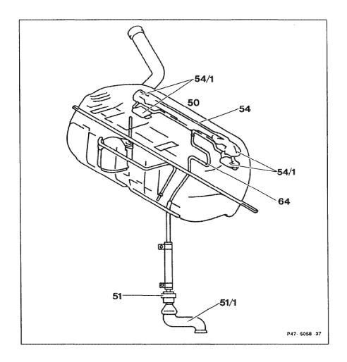
The vent system consists of a central pipe (54) with interrupt vessels (54/1) at the ends. The interrupt vessels (54/1) prevent fuel escaping along the vent line. The vent line (64) runs from the central pipe to the vent valve (51).
