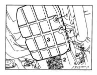
Turn crankshaft until drain plug (2) of torque converter is accessible through opening in vent grille. Remove drain plug and allow fluid to drain.
