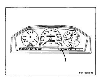
1 Exterior lamp failure indicator up to 09/85 in 1st field
