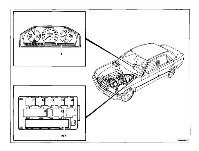
N7 Exterior lamp failure monitoring unit
