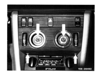
5 Remove screws, pull off electric plug connections and take off plate.
