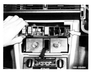
7 Unscrew nuts on connection from center console to instrument panel.
