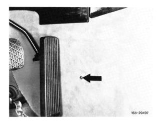
13 Disengage lower holding link of lateral tunnel lining.
