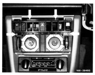
6 Pull off switch for heatable back window, push switch carrier to the right in forward direction out of detent and remove at the left toward the rear.
