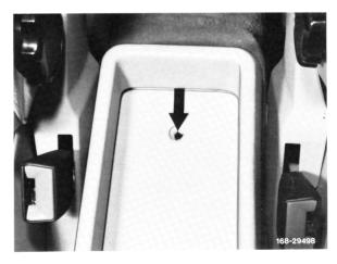
12 Unscrew front fastening screw left and right.
