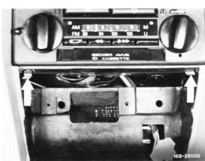
10 Push back detent and take switch plate out of holder.
