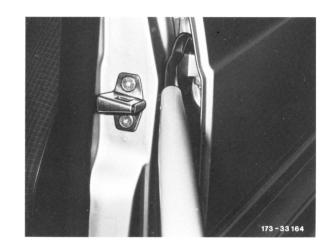
10 Insert centering gauge into door lock until the lock completely engages (detent stage 2).
