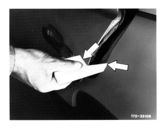
14 Check window frame in ranges A, B and C and straighten, if required.
