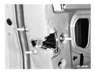
10 Insert locking cylinder with turning bar into turning socket on door lock and fasten.
