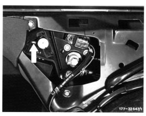
5 Pull off electric connection and unscrew tilting/sliding sun roof motor.
