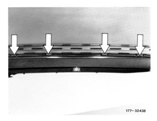
2 Unscrew tube on tilting/sliding sun roof frame, rear.
