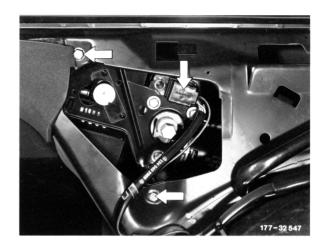
6 Disengage tube on tilting/sliding sun roof motor and remove tilting/sliding sun roof motor.
