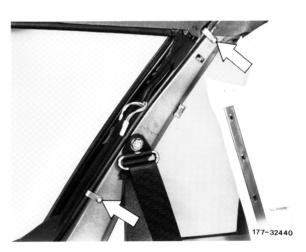
4 Disengage outlet tube on tilting/sliding sun roof motor, remove from clips at the rear and take off.
