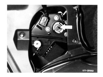
3 Unscrew fastening screws on holder and pull off electrical connection on sun roof motor.
