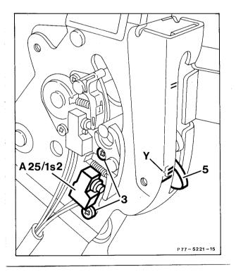
Unlock lock, connect multimeter to plug connection (A25/1x1, pins 1 and 2). Set multimeter to continuity test (acoustic signal). Press lock in direction "lock" with soft top key (vehicle tool kit). Simultaneously press rotary catch (5) upward with thumb to eliminate play. The soft top compartment cover switch "closed" (A25/1s1) should switch when the upper edge of the rotary catch (5) is in the switching range (Z). Adjust by moving in oblong holes if required.
