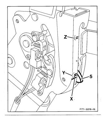
Unlock lock. Connect multimeter to plug connection (A25/1x1, pins 3 and 4). Set multimeter to continuity test (acoustic signal). Press lock in direction "lock" with soft top key (vehicle tool kit). Simultaneously press rotary catch (5) upward with thumb to eliminate play. Soft top compartment cover switch "locked" (A25/1s2) should switch when the upper edge of the rotary catch (5) is in the switching range (Y). Adjust by moving in oblong holes, if required.
