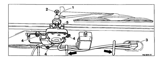
open, close. Hexagon nut (2) ...... unscrew, screw on. Wiper arm ...... take off, fit on. Cable straps (arrows) ...... open. Electrical connection (3) ...... unplug, plug in.
