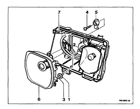
push back, fit on. Headlamp range control adjusting element (2) ... release by turning to the left, secure by turning to the right. Tie rod (3) of headlamp range control ....... detach from headlamp range control adjusting element (2), attach. Phillips screw (4) ..... unscrew, screw in. Holder (5) ...... take off, fit on. remove from mounting (7), replace. adjust lighting (82-1130). After installing headlamp unit ......
