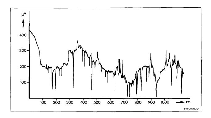
The field intensity diagram shows the pattern of such a field intensity. In a city, for example, signal differences up to a ratio of 1:1000 may occur within a few meters.
