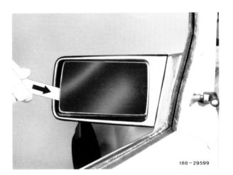
2 Position mirror glass against adjusting lever and force into mounting points.
