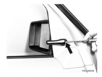
2 Unclip cover plate at top out of door frame and pull out of door trim in upward direction.
