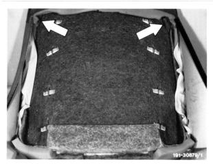
3 Cover both upper clips for retention in the longitudinal direction with large pieces of self-adhesive felt.
