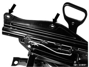
2 Grease oblong holes and adjusting mechanism on inclination adjustment shaft.
