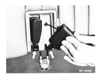
4 Slide trim on backrest hinge in upward direction.
