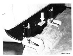
3 Expose belt locks at rear seat backrest, forcing off holder for this purpose and pulling elastic band out in downward direction.
