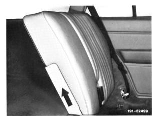
5 Unscrew screws (3 each) on backrest hinge.
