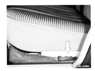
2 Pull up locking lever on underside of seat cushion and remove seat cushion in upward direction out of bearing pin.
