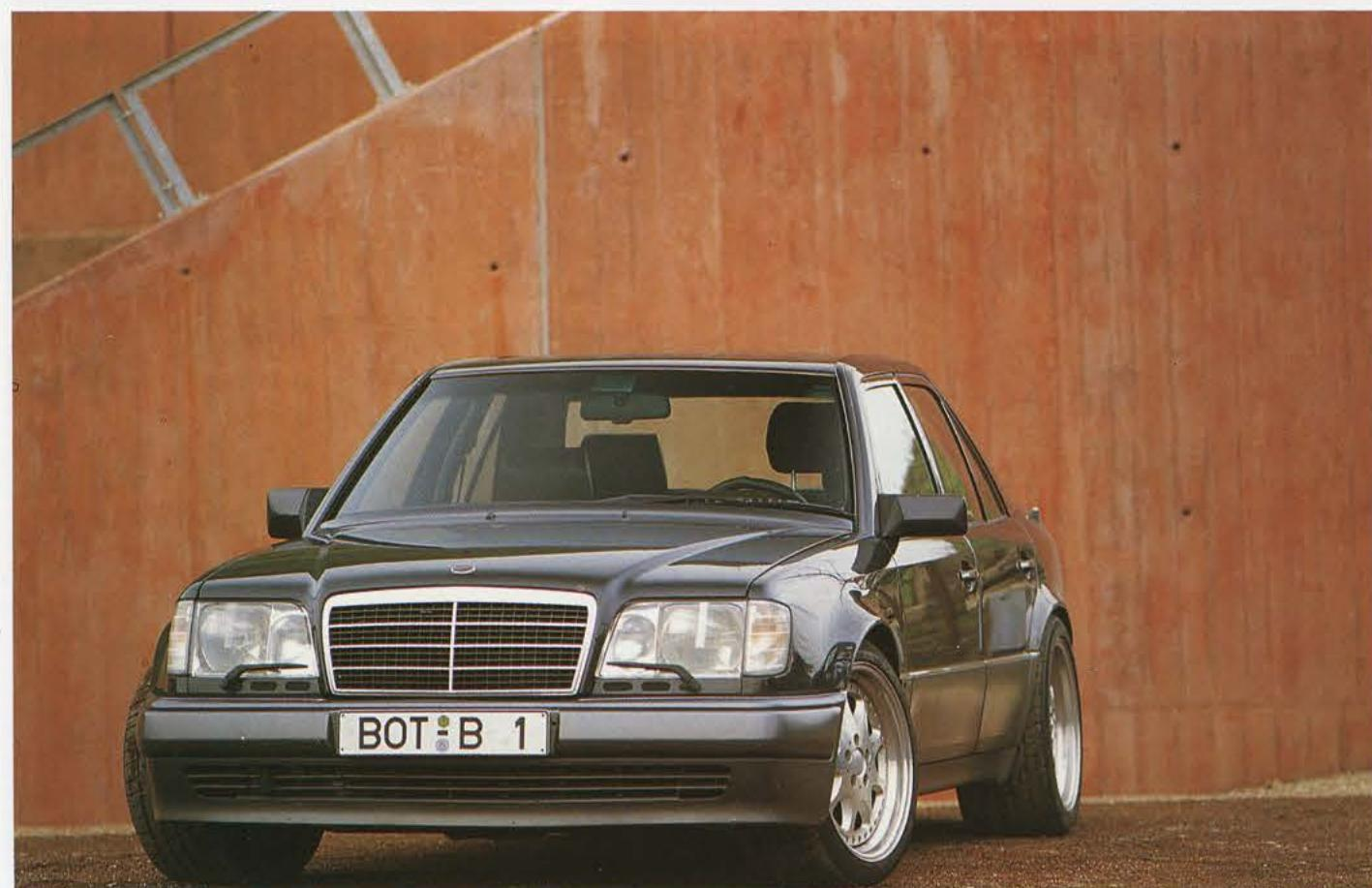
Transplanting their 7.3-48 engine into the Mercedes-Benz W124 E500, a car already acknowledged as a paragon of understated performance, BRABUS have produced the fastest four-door saloon in the world. With the power and torque of the consummate Mercedes-Benz sports saloon raised to 530 bhp at 5700 rpm and 755 Nm (557 ft lb) of torque at 3700rpm, it is a veritable sledgehammer, Arnold Schwarzenegger in an Armani suit!
